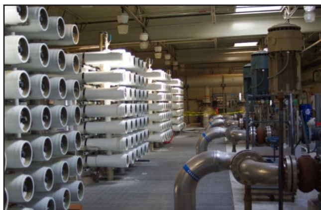
Figure 1. Four RO trains employing spiral wound membrane modules in Chino I Desalter (Chino, California).
