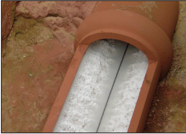
Figure 4. Precipitation in a brine line after 13 years in service at the Chino I Desalter. [16]
