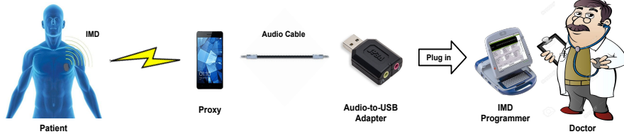
Figure 2: Architecture of Access Control with Audio Cable Connection
