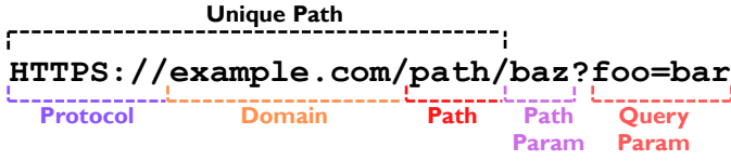
Fig. 2: Structure of a URL for example.com. Typically, parameters can be sent both in the URL and in the body of the HTTP request. We ignore the parameters to find the unique paths.
