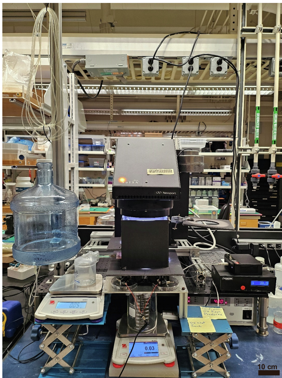
Figure S9. Image of the 1-day gravity-driven solar desalinator with convective cooling using v3-condenser. An air shield is constructed around the desalinator to prevent air flow from the fan reaching the evaporator.
