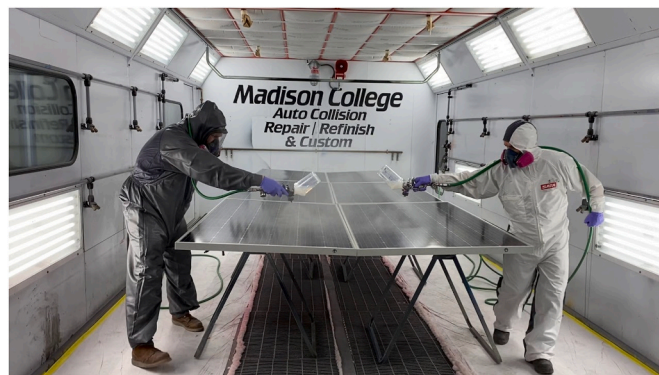
Fig. 3. Spray deposition of coatings in a controlled environment.
