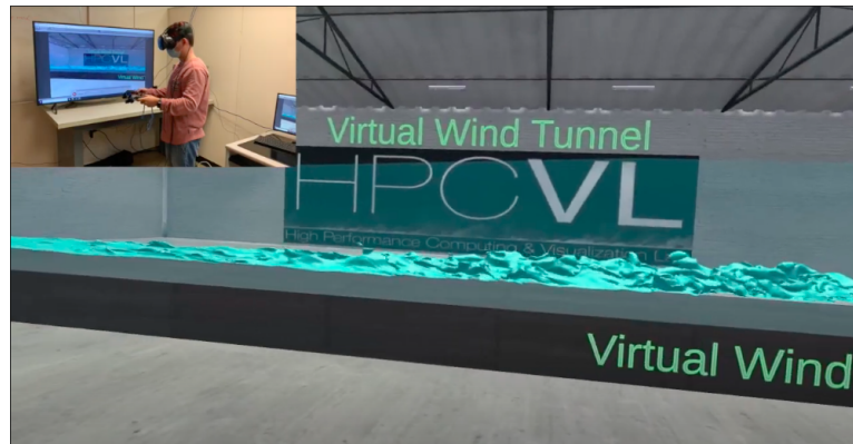
FIG. 8: User visualizing a flow in the VWT (iso-surface of instantaneous streamwise fluid velocity at 75% of the incoming freestream velocity, flow from right to left)
