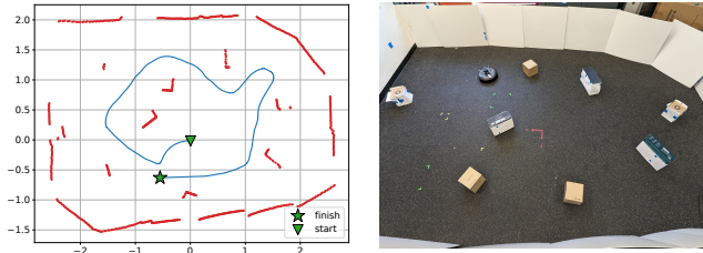
Fig. 3. Sample LiDAR scan and trajectory (left) and image (right) of the robot from the experimental setup.
