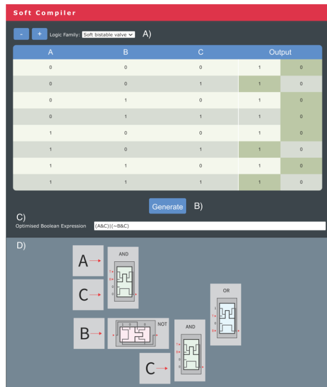
Fig. 1. The web-interface of the Soft Compiler. A) The user defines (1) the number of inputs to the soft circuit, (2) the soft logic family (here: “Soft bistable valve”) and (3) a truth table, mapping input combinations to a desired output response. B) Once the truth table is defined, “Generate” executes the compiler and outputs an optimized Boolean expression, and D) a schematic depicting the optimal wiring configuration that the user then implements during circuit assembly.
