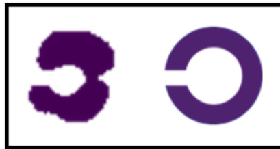
Figure 9. Optimized structure and split ring resonator (SRR) with similar parameters. The optimized structure had a significantly higher second-harmonic nonlinear optical response as compared to the split ring resonator.
