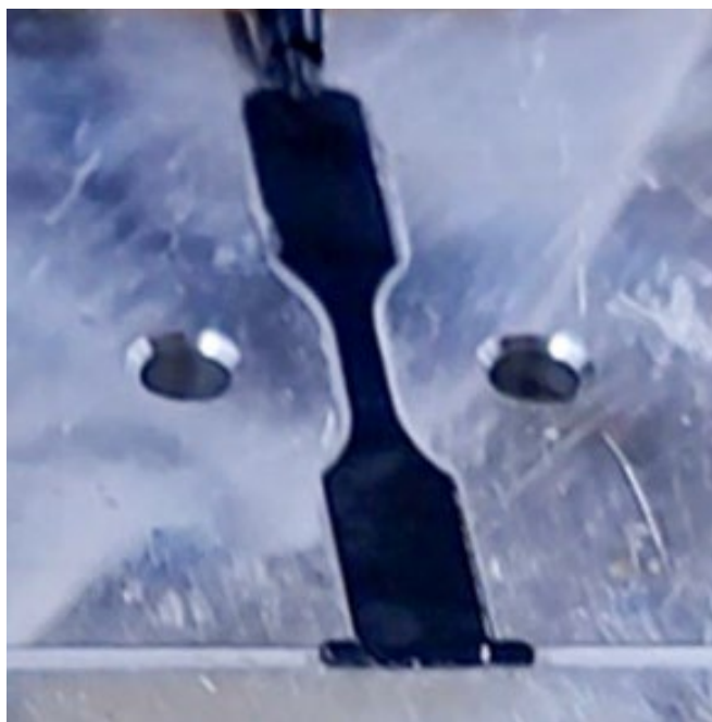
Figure S2. An injection molded ABS-matrix nanocomposite containing 0.1 wt% GSG.
