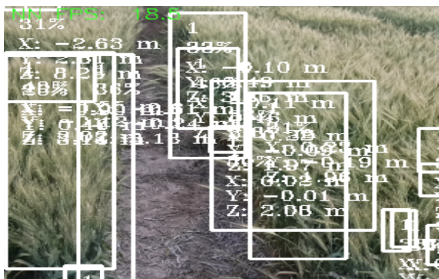
Figure 14. Real-time depth sensing of wheat in the field.
