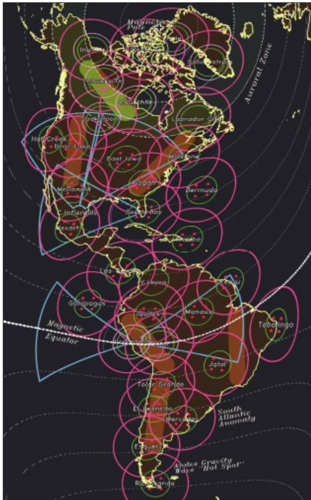
Figure 5: Fields of view (FoV) of the proposed observatories & instruments. Pink and green circles (projection distorted) indicate ground-based cameras imaging at 630 nm and 558 nm; four red dots indicate narrow-field FPI sampling; lilac circles denote SDI FoV; blue wedges show SuperDARN FoV; orange/green shadings denote the multistatic meteor radars FoV; and dashed contours show magnetic latitude.
