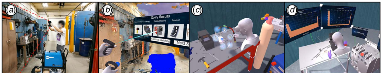
Fig. 1 Workflow of VRFromX (from left to right): (a) user scans a real environment to get the raw point cloud of the scene using an iPadPro, (b) user creates virtual content by interacting with the point cloud through AI assistance, (c) user attaches functions to the virtual objects using an Affordance Recommender, and (d) user interacts with the reconstructed scene in a virtual environment
