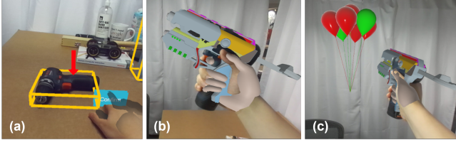
Figure 15: A demonstration of an AR shooting game with Ubi-TOUCH. The user wants a proxy for a virtual Nerf Gun and is suggested two proxies, a sprayer and a drill in the environment (a). The user's interaction with the drill is then mapped to the interaction with the Nerf Gun (b). The user then uses the drill to aim at some virtual balloons and shoot (c).
