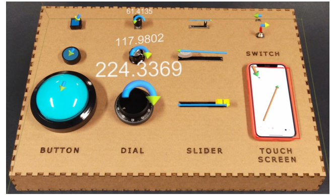
Figure 17: Mock-up machine for technical evaluation.
