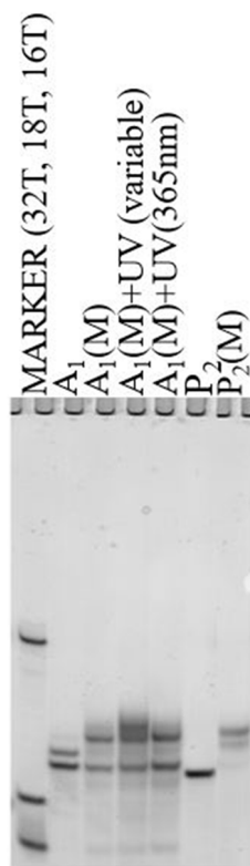
Figure 4. 20% native PAGE showing the modification of phosphorothioate backbone of the antisense strand ( A_1 ) and sense strand ( P_2 ) with TEEP-OH, and its subsequent photocleavage at two different wavelengths. The source of variable wavelength is the benchtop UV illuminator and 365 nm wavelength radiation was achieved using a 5860 filter with the benchtop UV illuminator.
