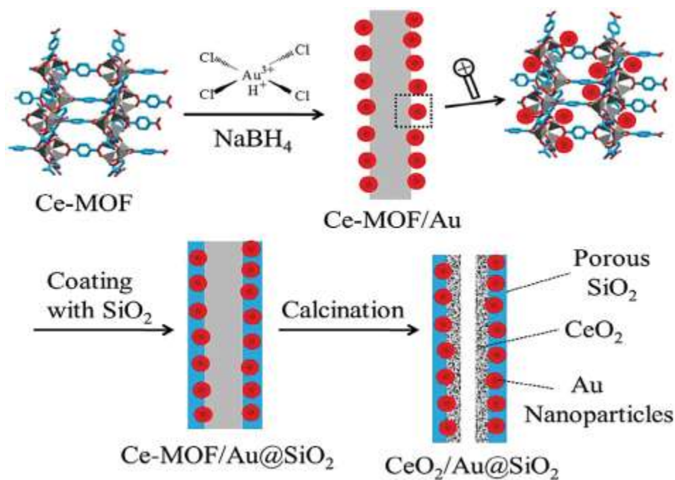
Figure 19. The synthesis procedure for \text{CeO}_2/\text{Au}@/\text{SiO}_2 nanocomposites. Reproduced from Ref. 299 with permission from the Royal Society of Chemistry.
