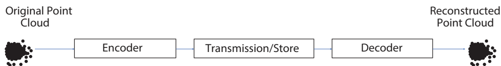
FIGURE 1. The general PCC system structure.
