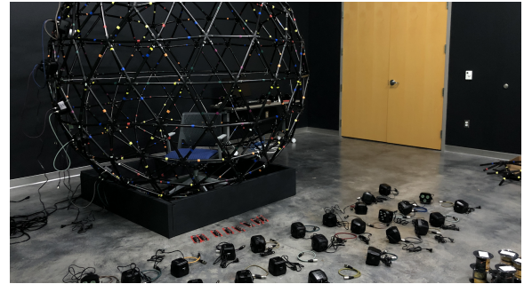
Figure 4: 4V geodesic kit from Sonostar assembled with systematic installation of lighting beginning.
