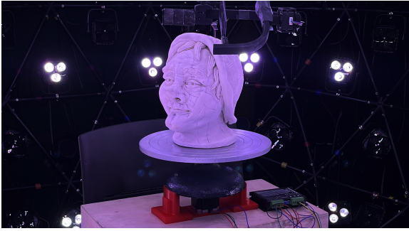
Figure 8: Sculpture on automated turntable, polarized illumination (viewing camera not cross-polarized here).
