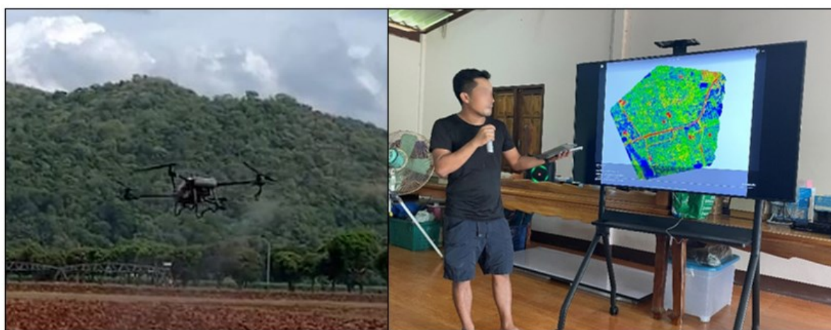
Figure 10. Left: A drone spraying pesticide. Right: Drone-captured NDVI of durian tree health monitoring, presented by a farmer. Photos taken in summer 2023 (credit: Gang Chen).
