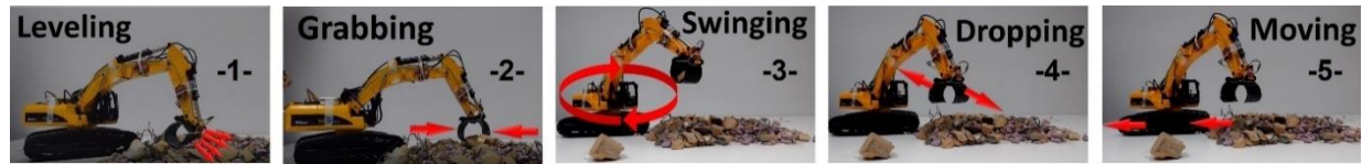
Figure 3. Classes of demolition waste material separation activities.
