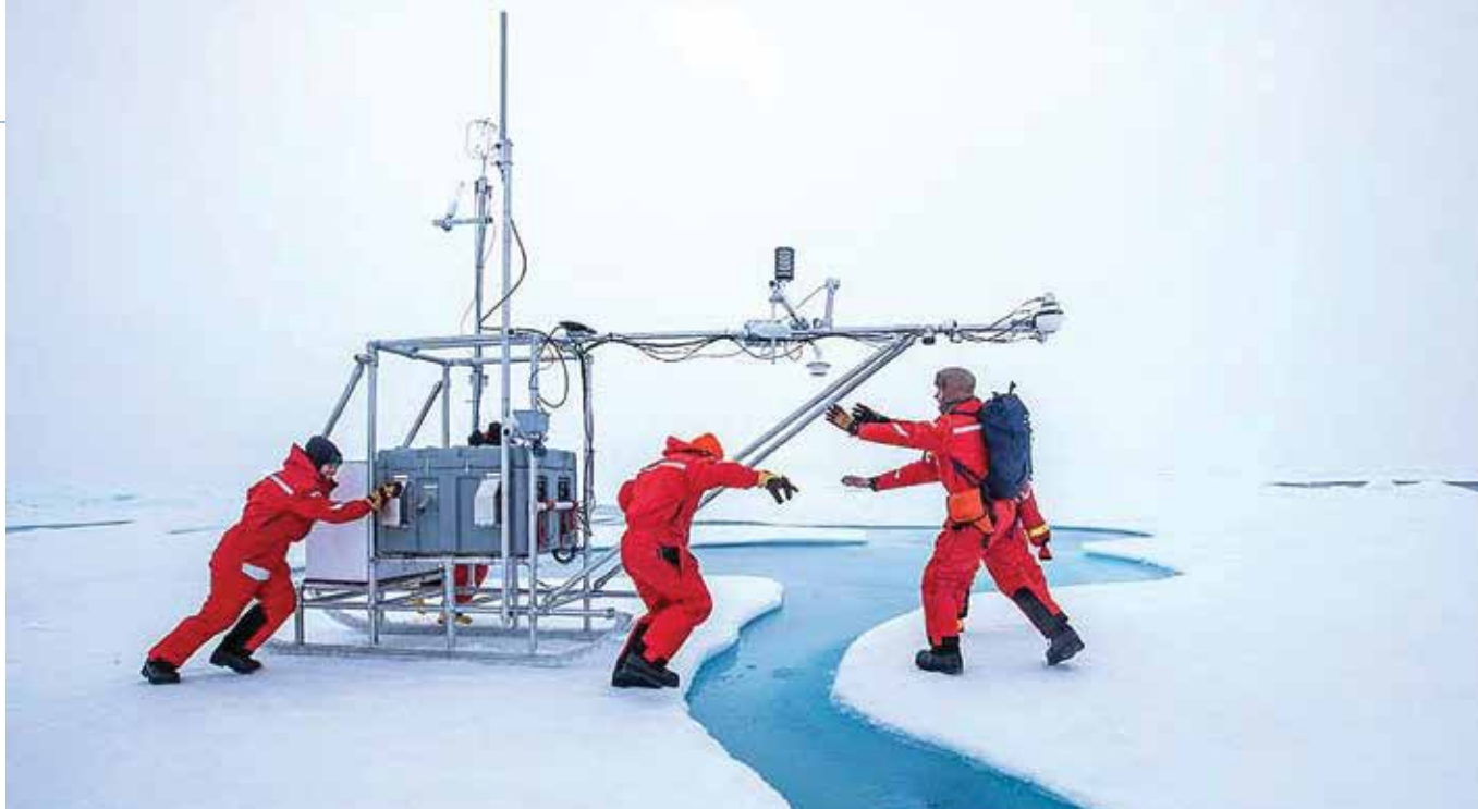
Scientists maneuver a “Flux Station,” a sled with instruments capable of measuring many atmospheric variables including temperature and radiation (incoming/outgoing), across the sea ice. Photo credit: Lianna Nixon
