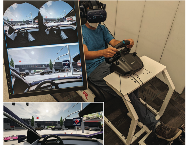
Fig. 1: Experimental setup showing a subject in our virtual reality driving simulator. The bucket seat and steering wheel and pedals help provide a realistic physical interface for driving. Red crosshair represents user gaze in the experimenter view, while it is not visible in VR to the user. Inset shows the experimenter view more clearly. Note the red sphere which serves as the peripheral stimulus that participants must respond to.
