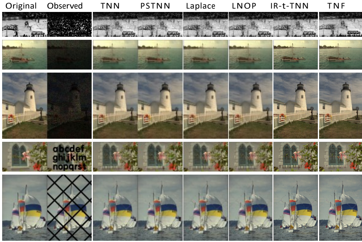
Figure 4. Comparison of video and image inpainting performance on five examples. From left to right: original image, observed input, recovered images by TNN, PSTNN, Laplace, LNOP, IR-t-TNN, and our TNF. From top to bottom: one frame of the video data ("basketball"), color images with random missing data ("sailboat1" and "castle"), and color images with structural missing data ("window" and "sailboat2").
