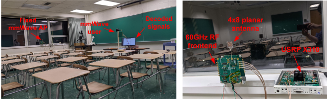
Fig. 3: Experimental setup in a classroom. Fig. 4: A picture of mmWave AP.
