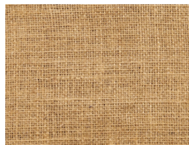
Figure 2. Woven jute textile used as reinforcements in this study.
