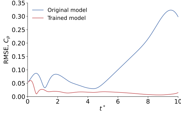
FIG. 7: Time evolution of root-mean-square error for C_p on the bottom wall. The unsteady-FIML-trained model significantly reduces the RMSE compared with the original model at all times.
