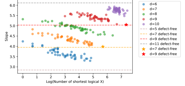
Figure 7. Slopes of LER v.s. p , from the same defective patches used in Fig. 5, grouped by d and plotted against the log of the number of shortest logical X.
