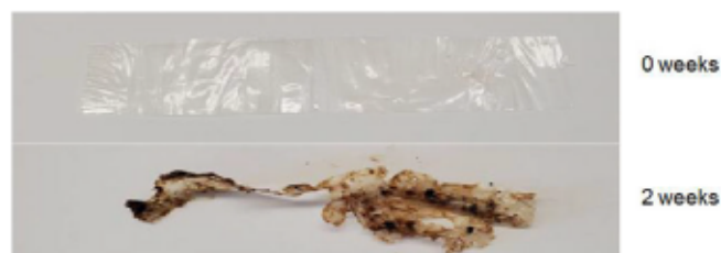
FIGURE 6 Polyhydroxyalkanoate-based clear sheet laminated with PUD 1 before compost (top) and after 2 weeks in compost (bottom). [Color figure can be viewed at wileyonlinelibrary.com ]
