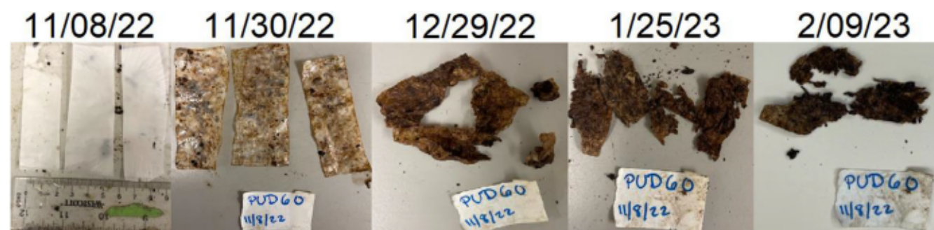
FIGURE 7 Progression of biodegradation of printed polyhydroxyalkanoate-based lamination with PUD 1 over the course of 3 months. [Color figure can be viewed at wileyonlinelibrary.com ]
