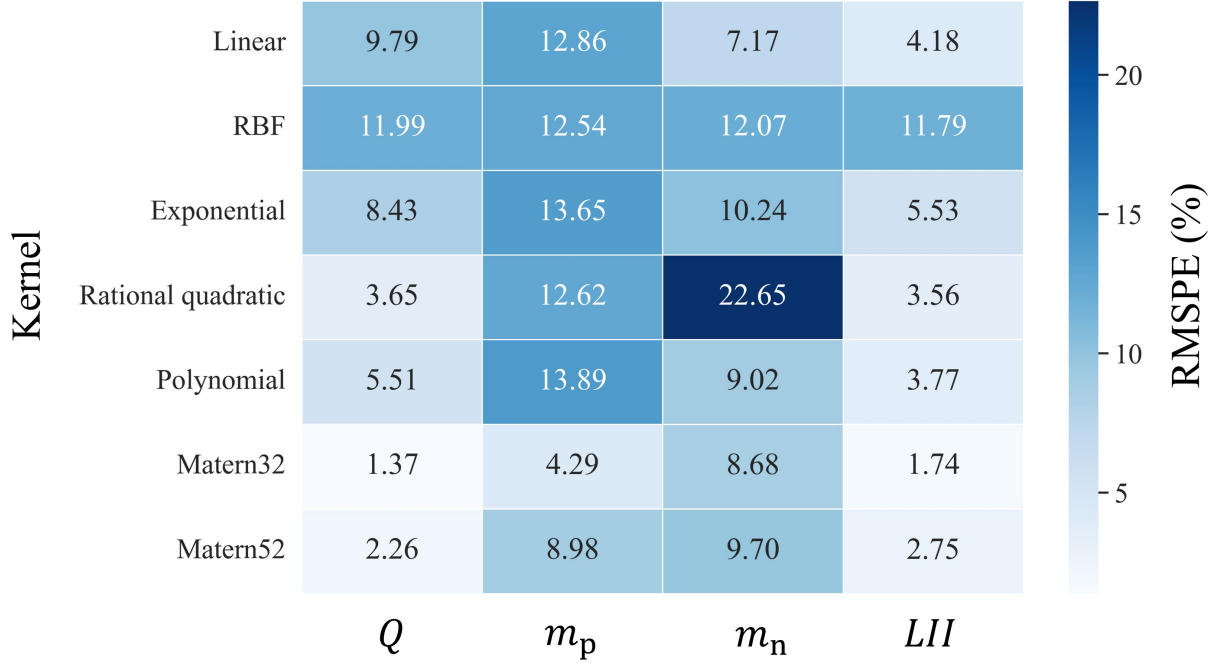
Figure 14: Sensitivity of prediction error rate of co-kriging model to different kernel functions
