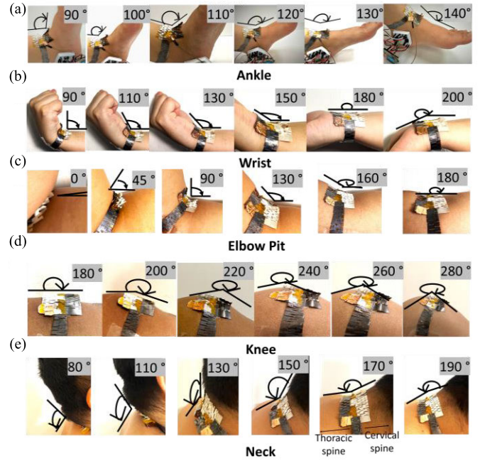
Fig. 11. Placement of sensors at the joints in (a) ankle, (b) wrist, (c) elbow pit, (d) knee, and (e) neck.
