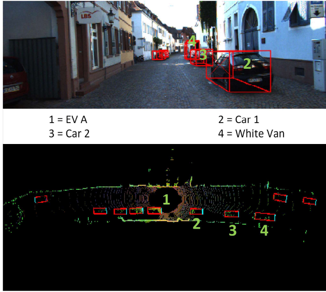
Fig. 6. Example case where the pedestrian is occluded from one vehicle's view but not the others'. The EV A is traveling in a straight road. The EV can detect the car 1, car 2, and the white van ahead. This frame is taken approximately 1.1 s earlier than Fig. 7, which makes the EV to be behind vehicle B in a real world scenario.
