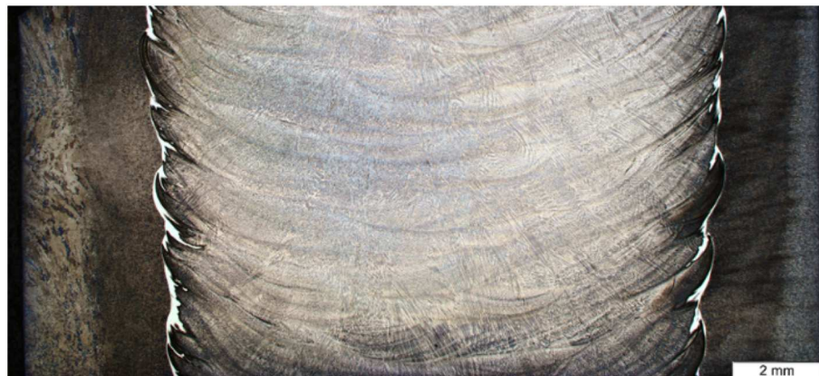
Fig. 3. Low magnification optical micrograph of the LAS butter weld (left) joined to the F65 steel pipe (right) using Alloy 625 filler wire.
