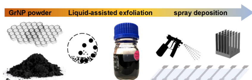
Scheme 1. Graphene nanoplatelet (GrNP) powder can be exfoliated by low-energy ball milling to form stable dispersions in pristine EtOAc or acetone, enabling its deposition as thin films and conformal coatings with rapid drying using conventional airspray equipment.
