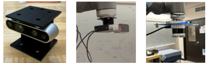
Fig. 1: The D435i, AKDK, and OS0 respectively in their mounts.
