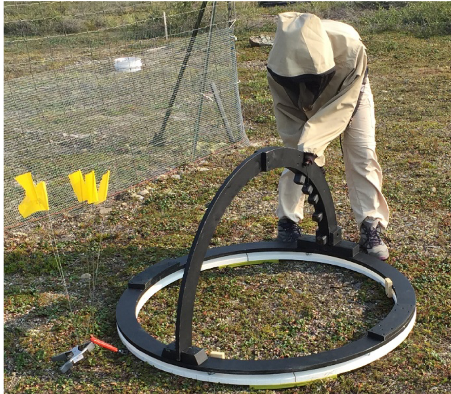
Figure 2. Photograph of camera and rig set up. The pin flags and clamp outside the base were used to indicate north. Five GoPro cameras were attached along the inner edge of the vertical arc. Photograph shows a control plot.
