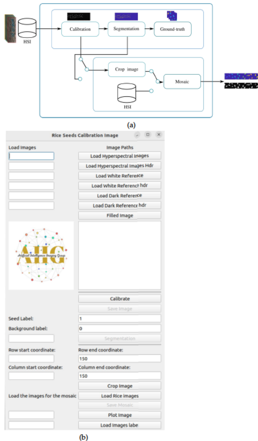
Figure 3. (a) Workflow for HSI seed images and ground truth mosaic construction, (b) HSI seed calibration application.
