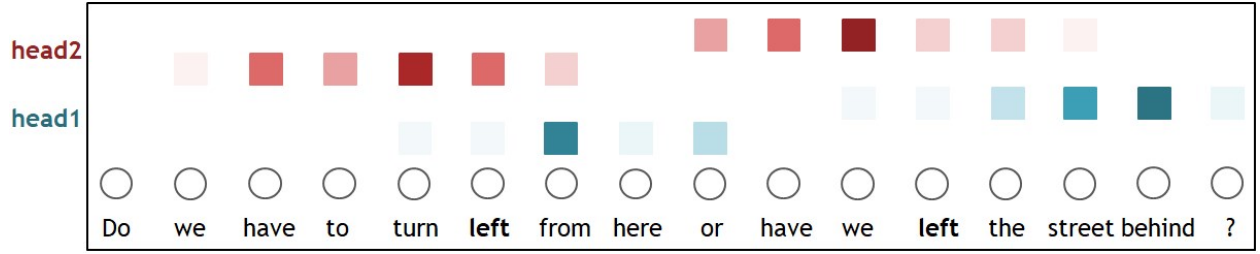
Figure 4: Multi-head self-attention example. Two heads can learn different attention weights for two different uses of the words “left” based on their meaning in the sentence. The relative attention weights shown are generated using the Transformer attention visualization tool [52].
