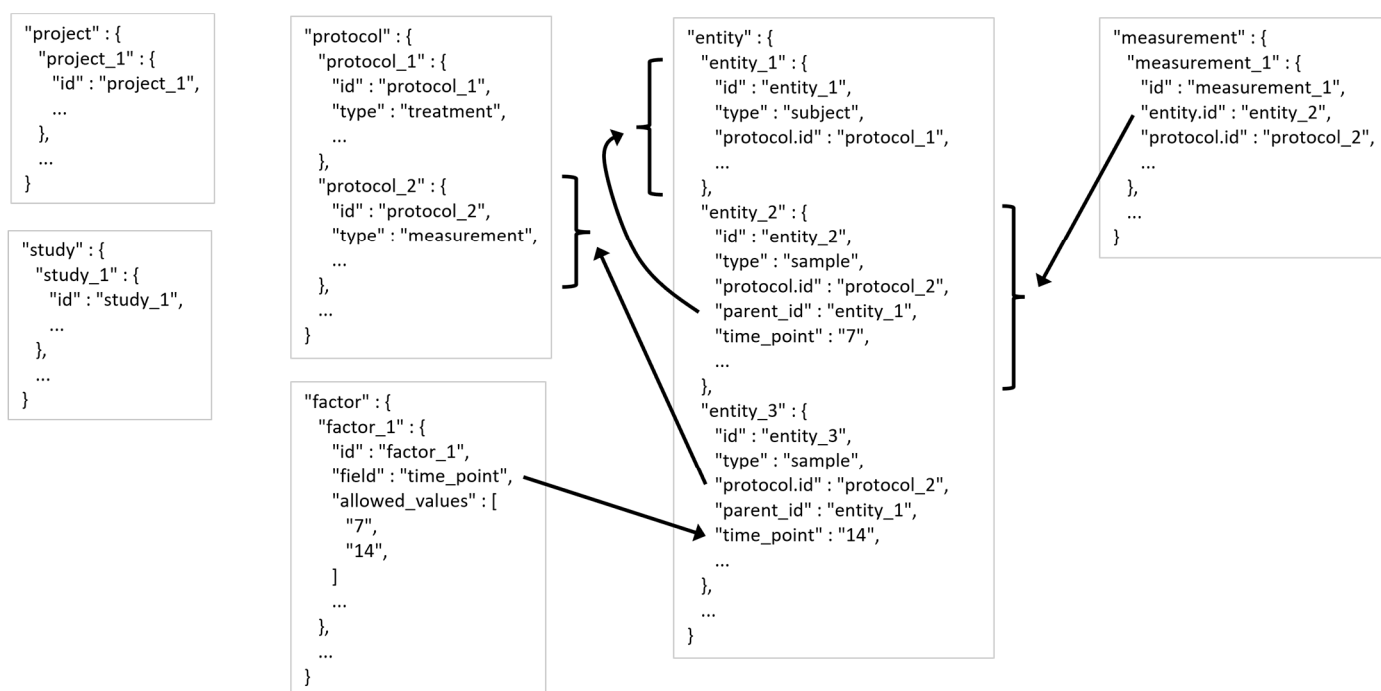
Figure 3. MESSES JSON Tables Example. Ellipses indicate that there could be more fields or records, while arrows point to records or fields that a field is referencing.
