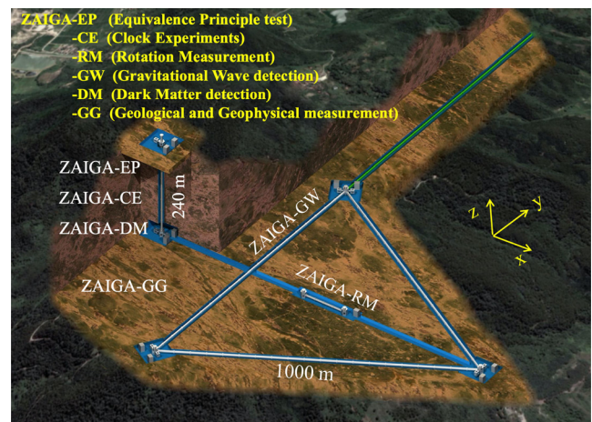
Fig. 22. Layout of the ZAIGA laboratory near Wuhan, China for a range of experiments using atom interferometry. Reproduced with permission from Zhan et al. , Int. J. Mod. Phys D 29 , 1940005 (2020). Copyright 2020 World Scientific Company.
