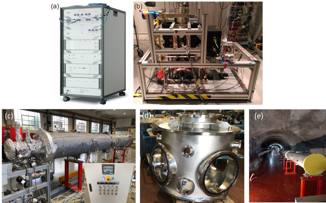
FIG. 20. (a) Fiber laser system developed by the Muquans company, reused with permission from Sabulsky et al. , Sci. Rep. 10 , 021101 (2020). Copyright 2020 Authors, licensed under a Creative Commons Attribution Unported License. 325 (b) cold ^{87}\text{Rb} atom source, reused with permission from Beaufils et al. , Sci. Rep. 12 , 231102 (2022). Copyright 2020 Authors, licensed under a Creative Commons Attribution Unported License. 267 (c) standard 6 m long section under vacuum test, (d) vacuum tower in production at SAES Parma (Italy), (e) MIGA gallery within the Laboratoire Souterrain à Bas Bruit (LSBB) and installation of the first sections of the vacuum vessel, reproduced with permission from Canuel et al. , “A gravity antenna based on quantum technologies: MIGA,” arXiv:2204.12137 . Copyright 2022. 326
