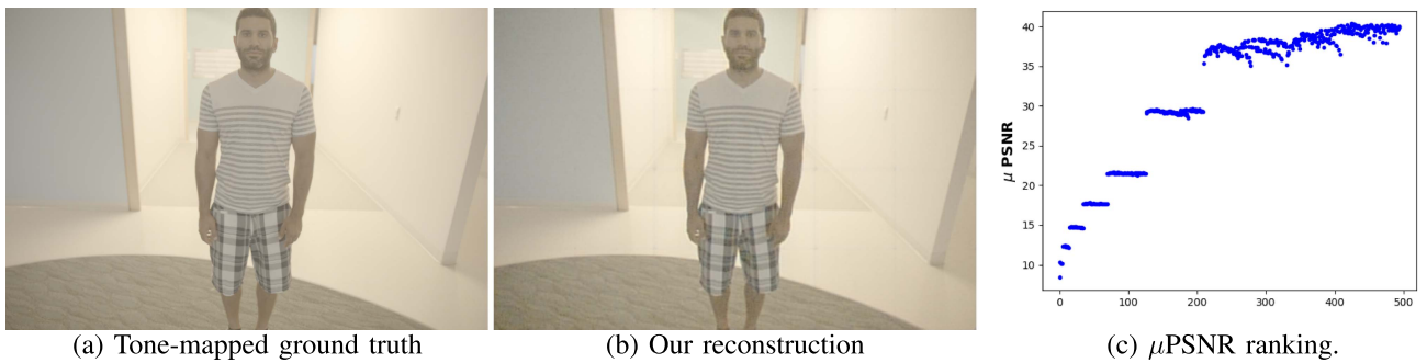
Fig. 13. Experimental results of SVE-Risk on color images. (a) tone-mapped ground truth, (b) tone-mapped reconstruction from the image captured with best pattern selected by SVE-Risk, (c) scatter plot of \mu PSNR as sorted from highest risk to lowest risk ranked by SVE-Risk.
