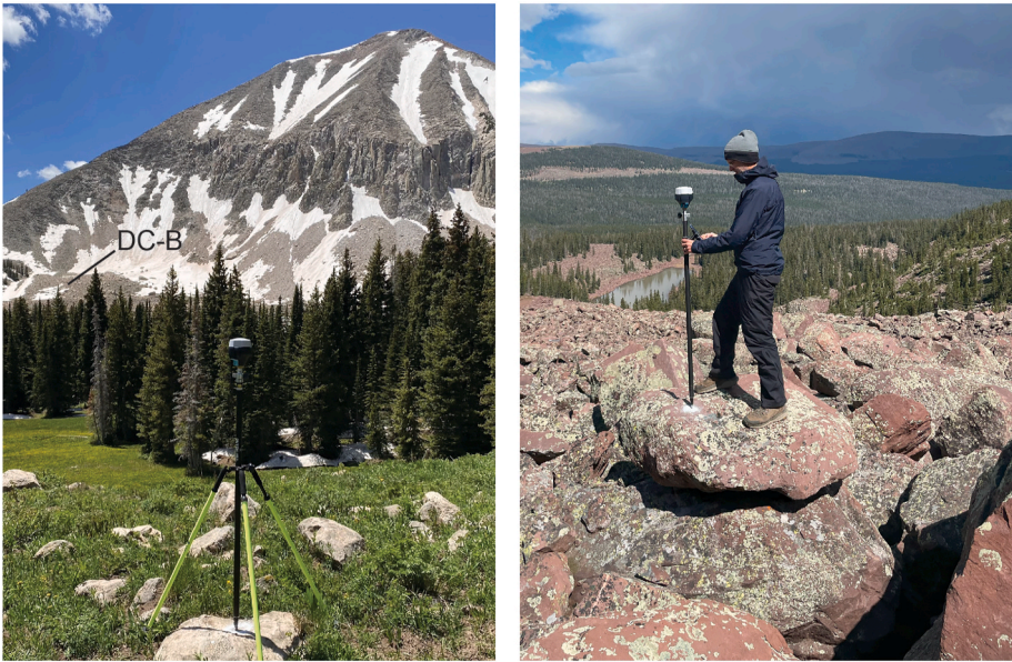
Fig. 3. Photographs presenting the field surveying methodology. Left image shows the GPS base station set up over a marked point on a stable boulder. Rock glacier DC-B is visible in the background (see Fig. 2). Right image shows the GPS rover measuring a marked point on the RG-2 rock glacier (see Fig. 2).
