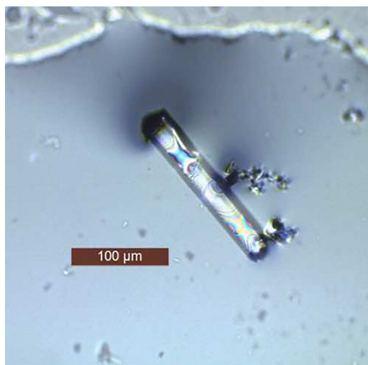
FIG. 3. A single crystal similar in transparency, shape, and size to what we picked for SXRD.
