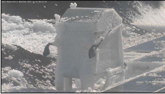
Figure 5. Webcam image of the SoCal enclosure frozen in a block of ice after a winter storm in 2022 December.
