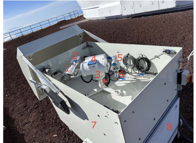
Figure 3. The SoCal tracker with mounted optics, inside its enclosure with the lid open. The numbered components are (1) Lens and lens tube, (2) Integrating sphere, (3) EKO Sun Tracker, (4) GPS sensor, (5) Pyrheliometer, (6) Sun-sensor, (7) Enclosure, and (8) E-box. The arrow indicates geographic north; i.e., the tracker is pointed south in this image.
