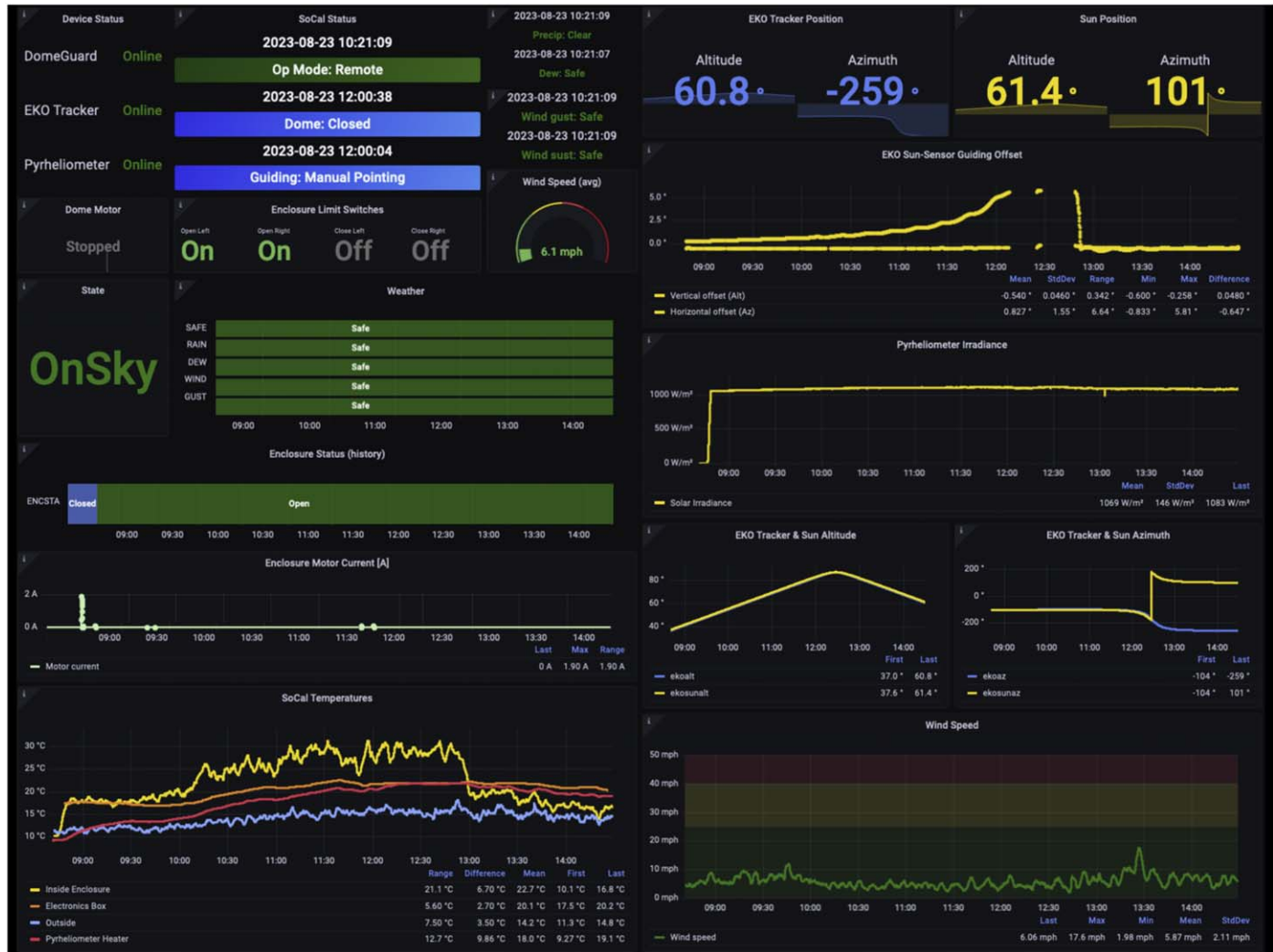
Figure 6. Screenshot of the Grafana web page displaying the SoCal telemetry for an example day. Grafana is a web-based interactive visualization software for displaying and plotting values from a database. In this example near the summer solstice, the tracker performed a large slew in azimuth through solar noon at near 90° elevations. The Sun sensor guiding offset is plotted in the upper right-hand corner (box titled “EKO Sun-Sensor Guiding Offset”). Near solar noon the Sun tracker switches to predictive guiding mode, hence the gap in recorded guider offsets. The elevation offset is stable at \sim 0.5^\circ \pm 0.05^\circ all day. While the azimuth offset increases near zenith, the actual angular separation between the predicted Sun location and the Sun tracker’s position is never more than \sim 0.5^\circ . Other panels display weather information and the status of subsystems.
