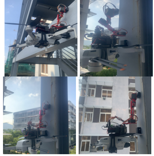
Fig. 14: Deployment of the robot on different locations for steel structure's data collection
