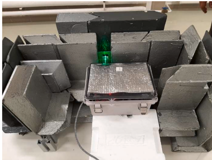
Fig. 7. Lead structure shielding the detector from the moving radiation source. The small 3 cm by 3 cm opening is shown by shining green laser light through it. This small opening allows the gamma-ray beam to pass without shielding when the moving radiation source is directly in front of the detector.
