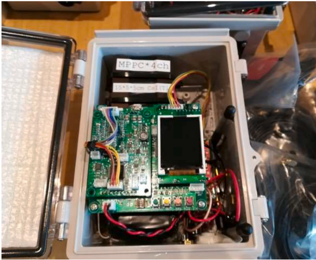
Fig. 2. Prototype Cesium Iodide scintillator-based Gamma-ray detector that has been deployed on commercial aircraft. The current data acquisition system uses time bins of 100 \mu s, and records photons from 300 keV to 10 MeV in five energy bins. Initial detector design and image provided by the University of Kyoto.
