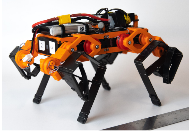
Fig. 1. Picture of the quadruped robot with tunable compliant laminate legs.
