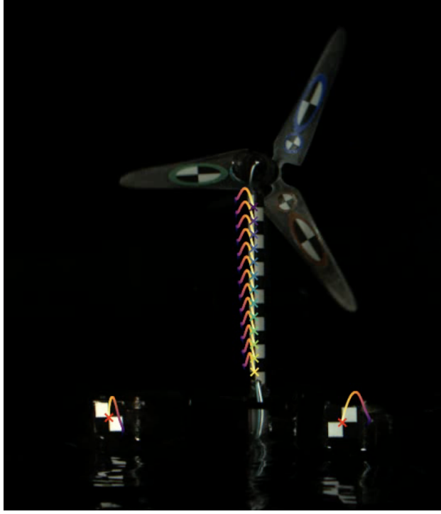
FIG. 4. Camera snapshot used for optical tracking, with indication of tracked markers and their previous trajectory for an incoming hub wind speed of 2.9m/s and a 1.2Hz wave conditions.
