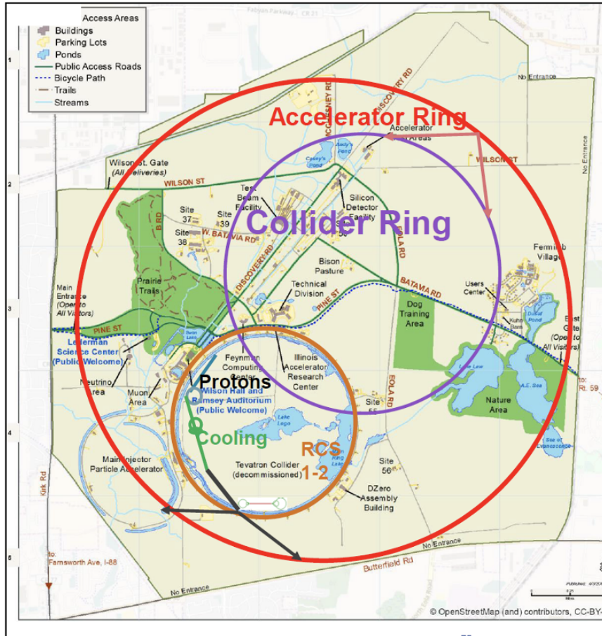
Figure 21. A schematic view of the Fermilab site and the layout of a possible complex for the Muon Collider. The protons start at PIP-II and are accelerated, bunched and pulsed onto a high power target. Muon cooling chain is indicated in green. Acceleration happens in stages with the final stage taking place inside the large Accelerator Ring. Muons at the nominal energy are injected into the Collider Ring, where the experiment(s) are located.
