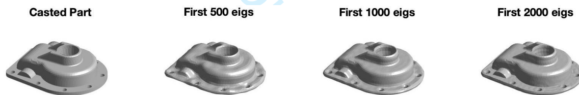
Figure 2 Approximated meshes of a casted part using the first 500, 1000, and 2000 eigenvectors, respectively.
